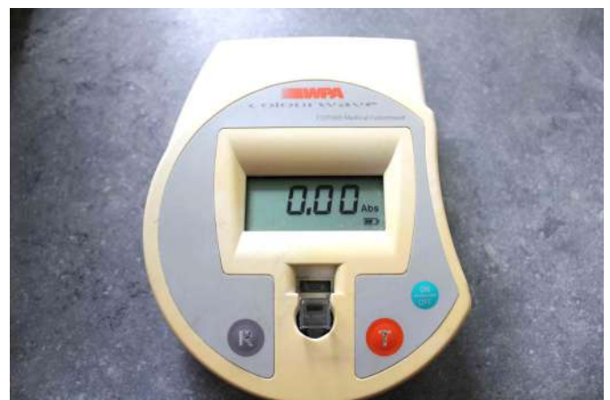
Figure 7.3: A colourimeter, used to measure the turbidity of the solution in the Zinc Sulphate Turbidity Test. Photo: Ian Hogan.
